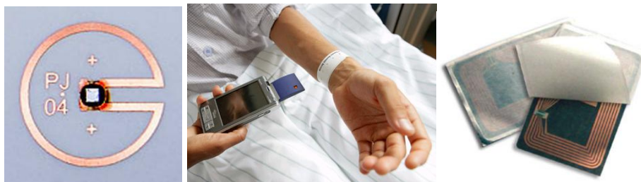
FIG 7. Transponder antennas are of small size and have stringent manufacturability and cost constraints. Typically the conductors are screen printed onto a flexible substrate.
