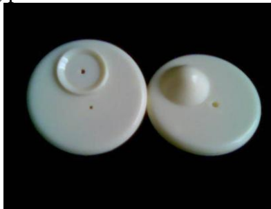
FIG 10. Reusable hard tag transponder antennae are more expensive to produce but can contain antenna coils of many windings. This increases the mutual inductance of the reader and transponder antenna system and increases the read range, or reduces the current requirements of the reader antenna.
